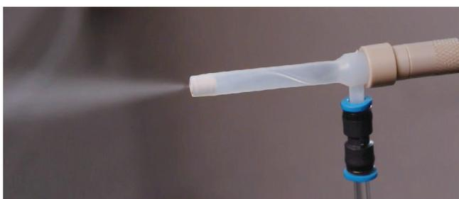
The Agilent nebulizer cleaning tool cannot be used for backflushing the Agilent OneNeb nebulizer as it differs in construction to concentric nebulizers.
